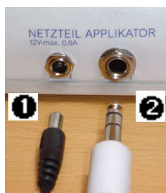
Circuit points: 1 Wall power supply, 2 Magnetic field therapy mat
